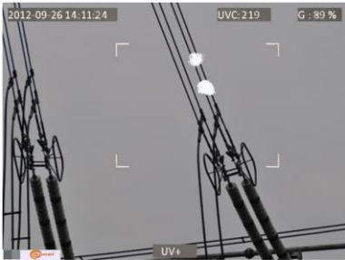
Fig. 3, 4. Corona discharge in laboratory conditions.
