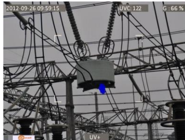
Fig. 5-8. Corona discharge in real power grids.
