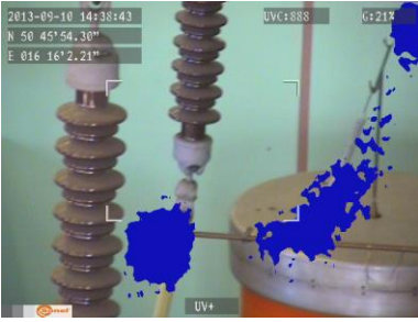
Fig. 3, 4. Corona discharge in laboratory conditions.
